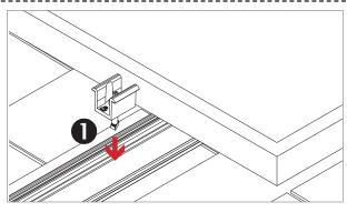
INSERT MIDCLAMP ASSEMBLY: Insert 1/4" T-Bolt into top slot of rail
