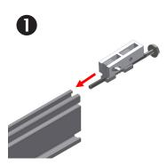
**INSTALL END CLAMPS ON RAIL:** Slide end clamp on to rail by engaging the two t-quide brackets with the top slot of the rails. **Ensure** bolt is extended as far as possible so that clamp is positioned at max. distance from end of rail.
