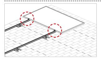
INSTALL MIDCLAMPS: Midclamp is supplied as an assembly with a T-bolt for module installation. Clamp assemblies may be positioned in rail near point of use prior to module placement.
