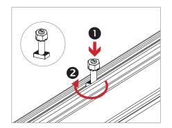
**INSTALL MICROINVERTER MOUNT T-BOLT:** Apply Anti-Seize and install pre-assembled ¼" dia. bonding T-bolts into top ¼" rail slot at microinverter locations. Rotate bolts into position.
