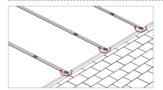
TRIM MIDCLAMPS: Ensure Trim lip is in contact with module face and verify alignment marks on T-bolts are in proper position, tighten midclamp on Trim, repeat at each gap between modules.
