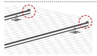
**INSTALL MODULE END CLAMPS:** The Fnd clamp is supplied as an assembly with a 1/2" hex head bolt that is accessible at the ends of rails. The clamp should be installed on the rails prior to installing end modules.
