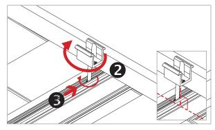
MIDCLAMP: Rotate midclamp assembly and slide until clamp is against module frame. Do not tighten nut until next module is in position. Ensure bolt is perpendicular to rail.
