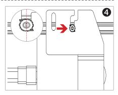
**ALIGN POSITION INDICATOR:** Verify that position indicator on bolt is perpendicular to rail.
