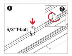
**PLACE T-BOLT INTO RAIL & SECURE BOLT:** Insert 3/8" T-bolt into rail at
