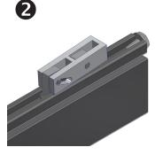
**POSITION END CLAMPS:** Slide end clamp assembly on to rail until bolt head engages with end of rail End clamps are positioned on rails prior to the first end module and prior to the last end module.
