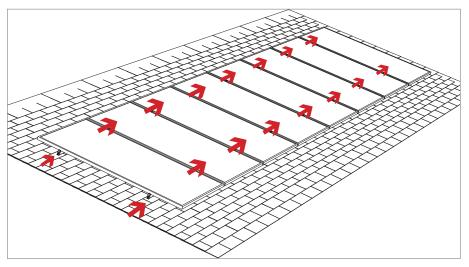
**FINISH MODULE INSTALLATION:** Proceed with module installation. Engage each module with the previously positioned clamp assembly:
