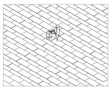
**DRILL PILOT HOLES:** Center the roof attachment over the rafter and drill a pilot hole(s) for the lag bolt(s).
