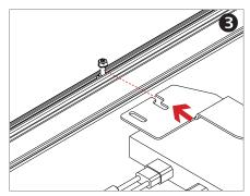
**INSTALL MICROINVERTER:** Install microinverter on to rail. Engage with holt
