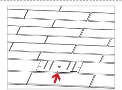
FLASHING INSTALLATION: Insert the flashing so the top part is under the next row of shingles and the hole lines up with the pilot hole.
