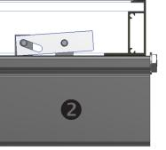
**ENGAGE CLAMP:** While holding module in position and with flange in full contact with rail, rotate end clamp bolt until clamp engages with flange to provide clamp force.
