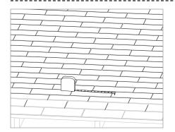
**ROOF PREPARATION:** Layout and install flashing at rafter locations determined per Design and Engineering Guide.
