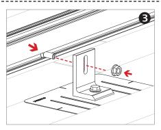
**SECURE T-BOLT:** Apply Anti-Seize to bolt. Rotate T-bolt into position.
