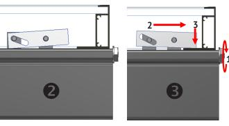
ENGAGE CLAMP: While holding module in position and with flange in full contact with rail, rotate end clamp bolt until clamp engages with flange to provide clamp force. To ensure bolt is not over-torqued, use low torque setting on drill or If using an impact driver, stop rotation as soon as impact action of driver begins.
