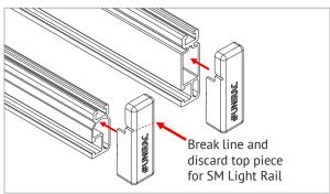
**INSTALL END CAPS:** End caps install as supplied on SM standard rail and SM light rail. If desired for SM light rail, the end cap may be modified as shown by hand, or by using a cutting tool.
