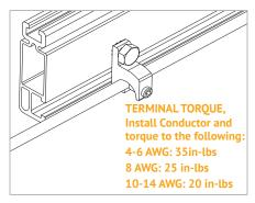
ILSCO LAY-IN LUG CONDUCTOR - UNIRAC P/N 008009P: Alternate Grounding Lug
