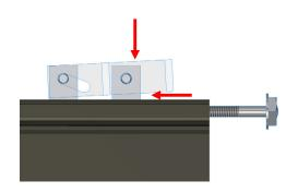
NOTE: To assist insertion of clamp into rail slot, Pressure may be applied to top or side of bracket as shown. Do not force clamp into rail by pushing on bolt with excessive force.
