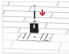
**INSTALL LAG BOLTS & L-FOOT:** Insert the lag bolt through the L-Foot in the order shown in the illustration. Verify proper orientation before
